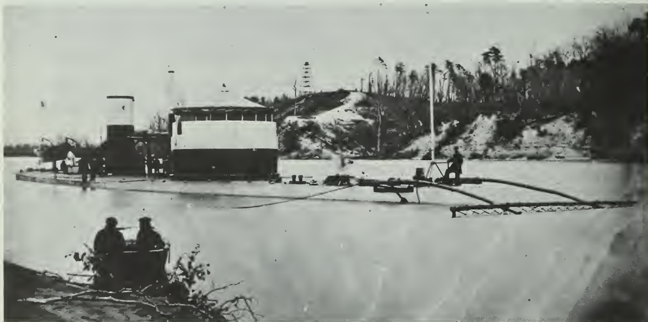
U.S. Monitor Saugus on the James River during the Civil War—The booms and netting protruding from the bow of Saugus are a so-called "torpedo rake", designed to sweep Confederate mines from the path of the ship.
